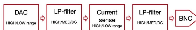
Figure 4. Key function blocks of each channel on QDAC-II: D/A converter with two ranges, low-pass filtering with three cut-offs, and current sensing with two ranges.
