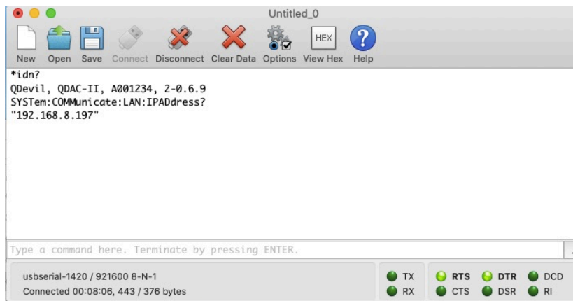
Figure 9. Example of sending a few commands via CoolTerm on a Mac.
