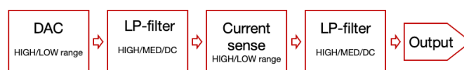
Figure 4. Key function blocks of each channel on QDAC-II Compact: D/A converter with two ranges, low-pass filtering with three cut-offs, and current sensing with two ranges.
